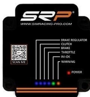
**POWER:** Red Led indicating that the plate is powered by USB.
